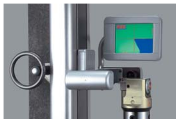
Display of angular grid (1 degree increment) for inspection of Tool cutting edge
