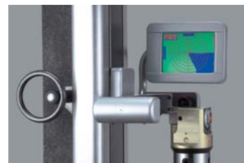
Display of reference circles for measurement of Nose Radius.
