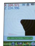
Nose R of the cutting edge (Concentric circle by each 0.2mm)
