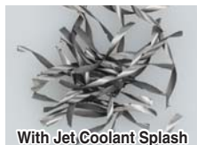
With Jet Coolant Splash
